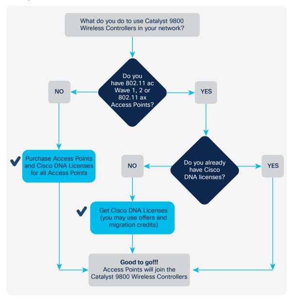
Access points connecting to a Cisco Catalyst 9800 Series controller have new and simplified software subscription packages.
