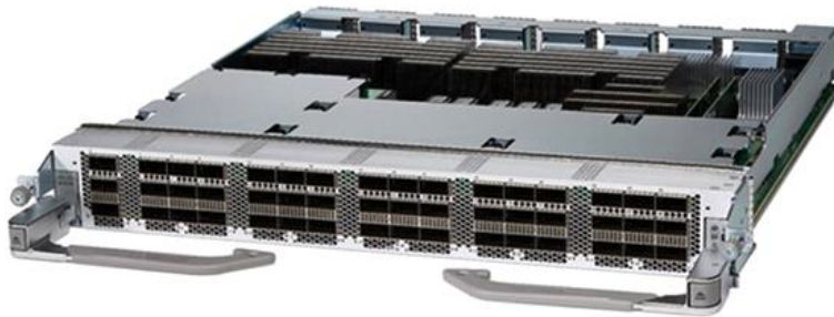
Figure 12. 48-port QSFP28 100GbE line card
