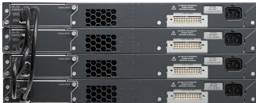
Figure 5. Cisco FlexStack-Plus switch stack
